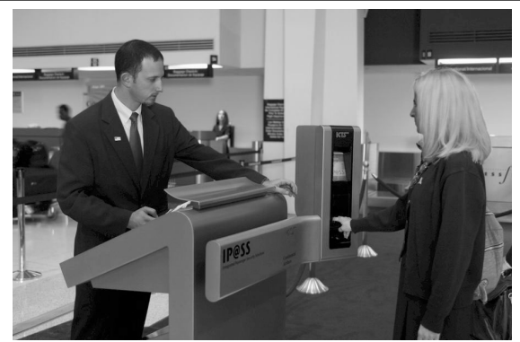
Passengers using the IP@SS reservation system provide two-finger 3-D geometry samples as their biometric identifier at Newark Airport during check-in.
