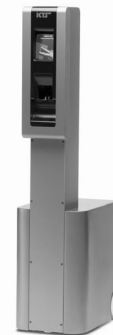
At the gate, passengers pass their contact-less smart card by the reader on top of the unit and place two fingers into the biometric reader in the middle of the unit.
